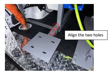
• Secure the VISE MOUNTING PLATE WILTON (02R656) to the tube using the provided Knob.
