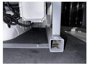
• Insert the (1) VISE MOUNTING PLATE WILTON (02R656) into the tube. Align the first hole on the vise mounting plate with the hole on the tube.
