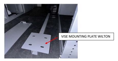
• A Vise Mount Tube to hold the Vise Mount is located at the base of the Compressor Stand. It is welded to the stand.
