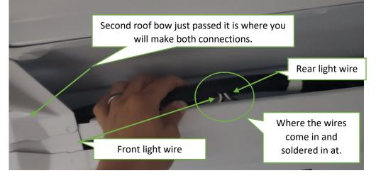
• Carefully locate the wires that you will be soldering into. Red with a green trace and which will connect to the black wire you ran. Then locate the white wire in the harness and connect it to the white wire you ran.
