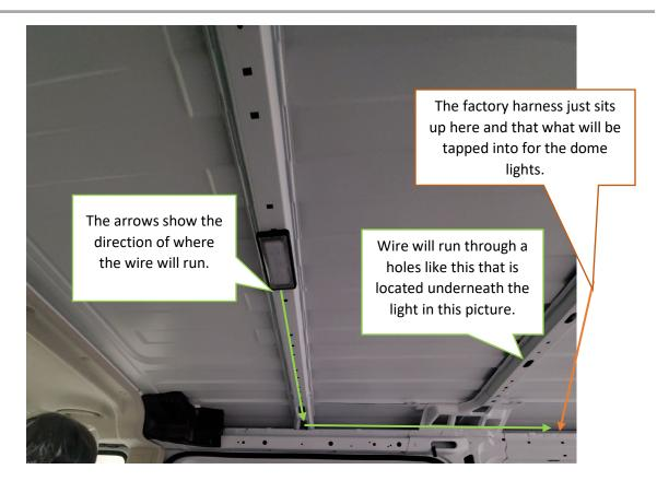
• The main harness of the van runs top side of the passenger side of the van. This is where the wires will run out to and be soldered into the van.
