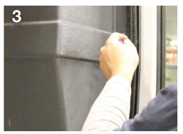
Using the pre-drilled holes in the partition as a guide, mark the holes at the end of the steel rib on the B-pillars. Remove the partition. Drill pilot holes through the plastic and the metal B-pillar.
