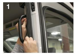
Pull back the rubber trim from around the door frame. Then remove the pillar handle. Remove the D-rings.
