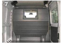
Adjust the weatherstripping trim along the door frames. The rubber should cover the outer edge of the panel. Installtion is complete.
