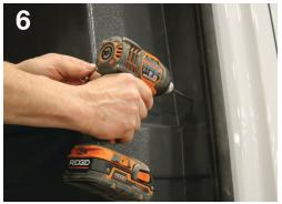
Using self-drilling screws (**F**), loosely secure the rest of the partition in the pre-drilled holes of the partition. When properly positioned, tighten all bolts.
