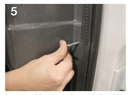
Insert partition. Loosely attach the sides of the partition with the 2" screws (**A**), washers (**C**), and split washers (**D**). Replace the D-rings.
