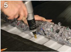
Insert plus nuts (**B**) using the plus nut gun. Insert the spacers (**A**) in the 1" hole of the B-pillars plastic.
