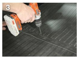
Pull back the carpet and trim the felt padding by 3". Cut holes through the carpet where it is marked.
