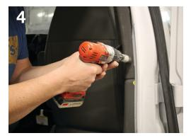
Drill pilot holes through the plastic and the metal B-pillar, and in the floor. Using the 1" hole saw, cut the B-pillar plastic as marked. Drill a 11/32" in the B-pillar metal and in the floor. Refer to diagram on next page.
