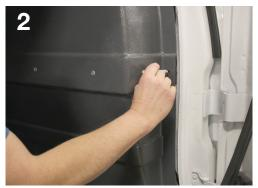
Mark the holes in the bottom bracket of the partition and mark the holes in the steel rib of the partition aligned with the B-pillar. Remove the partition.
