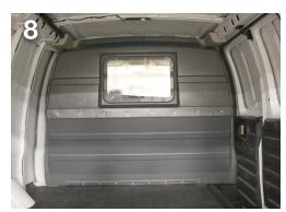
Adjust the weatherstripping along the door frames. The rubber should cover the outer edge of the panel. Installation is now complete.
