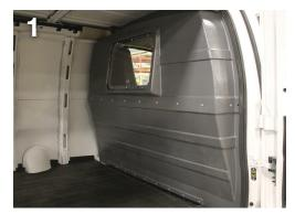
Pull back the rubber trim from around the door frames. Slide the partition into place so that it lines up against the B-Pillar and along the headliner.
