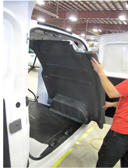
Slide the panel in through the rear doors at an angle and position it on the wall. The panel will fit with the contour of the van.
