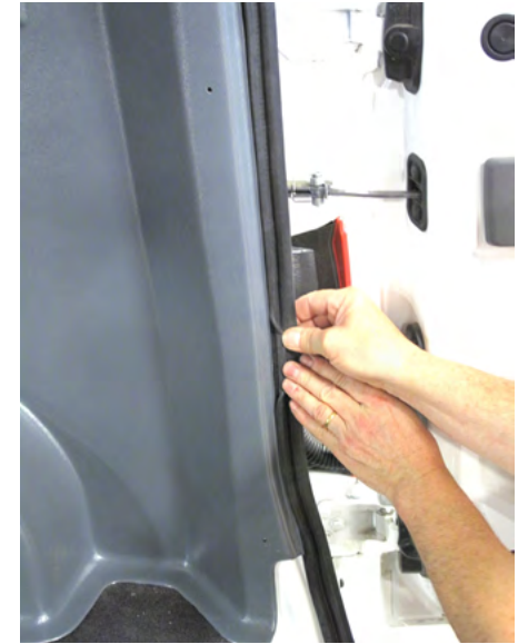
Re-attach the weather stripping – cover the edge of the wall panel with it as shown.
