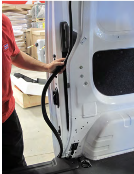
Pull back rubber weather stripping from rear and side doors.
