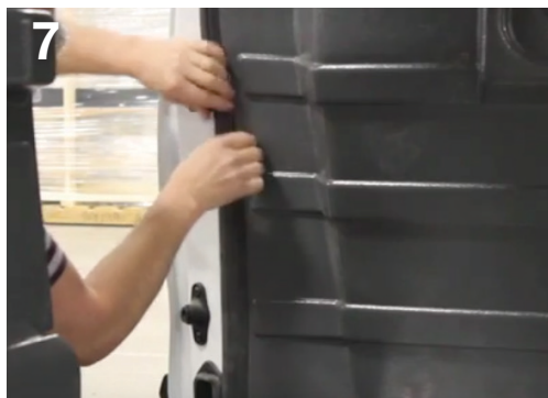
7 Adjust the weather stripping.
