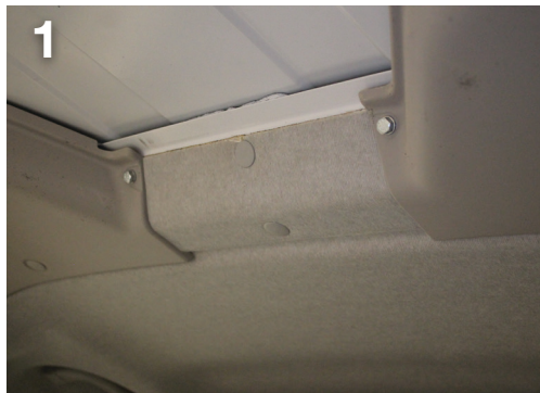
1 Remove 2 OEM bolts in headliner.
