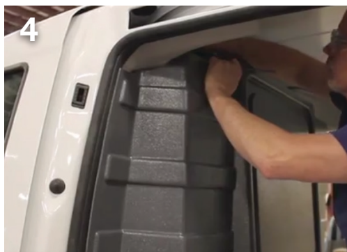
4 Loosely insert bolts (A) and washers (B) at the top of the partition.
