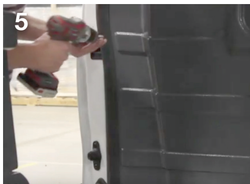
5 Loosely insert the self-tapping screws (C) in the remaining pre-drilled holes on the side of the partition.
