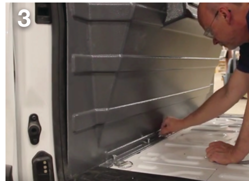
3 Loosely insert washers (D) and bolts (E) at the bottom of the panel to secure the floor plate to the van floor.
