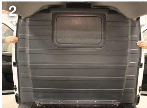
2 Slide the partition panel into place so that it lines up against the B-Pillar and along the headliner.
