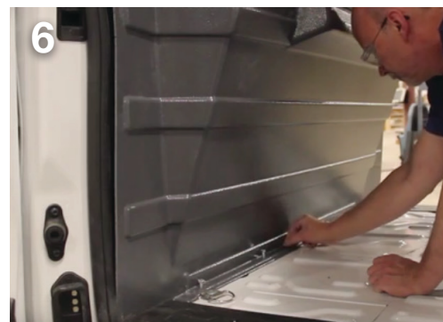
6 When properly positioned, tighten all bolts.
