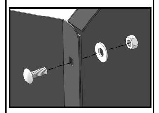
Align holes in Left Panel as shown and secure using:
