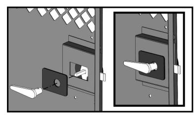
Attach the Plastic Latch Cover Plate and the Chrome inside Handle firmly to the back of the Round Handle. Be sure the inside handle is parallel to the floor, but facing the opposite direction of the locking mechanism.
