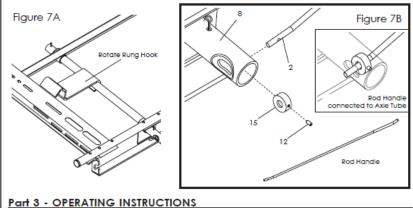
In the UNLOCKED position, the ROD HANDLE should be securely seated in the forward position of the HANDLELOCK.
