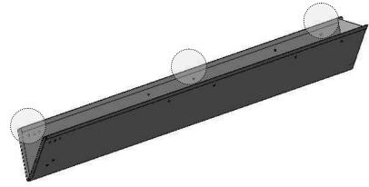
Place Troughs in vehicle to mark (3) mounting locations along the street side if the van as shown preferably at Pillars. Mark locations and install 1/4 Plusnuts (See Fig 4)
