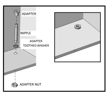
Insert bottom vent pipe through hole in cabinet floor as shown here.
