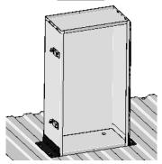
Position cabinet in desired location, and mark the mounting hole locations through the slots in the mounting flanges.
