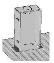
Drill a 3/4 hole in the top of cabinet to install top vent fitting.
