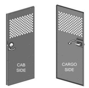
Once the handle is installed, turn clockwise to open from the outside, and counter clockwise to open from the inside.
