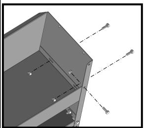
Attach Tool Drop Tray as shown, using: (6) 1/4-20 x 3/4 Hex Head Screws (6) 1/4-20 E-Stop Nuts
