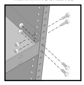
Attaching (2) HD Shelves as shown, using: (32) 1/4-20 x 3/4 Hex Head Screws (32) 1/4-20 E-Stop Nuts
