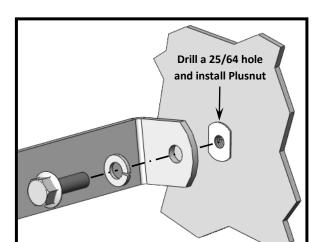
With module properly positioned in desired location in vehicle, attach brackets loosely at the locations shown. Mark and drill 25/64 holes to install Plusnuts and secure as shown using:
