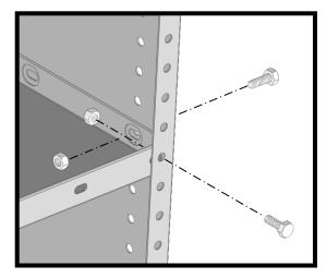
Attaching (2) Shelves as shown, using: (16) 1/4-20 x 3/4 Hex Head Screws (16) 1/4-20 E-Stop Nuts
