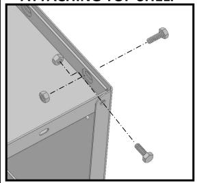
Attach Top Shelf as shown, using: (6) 1/4-20 x 3/4 Hex Head Screws (6) 1/4-20 E-Stop Nuts
