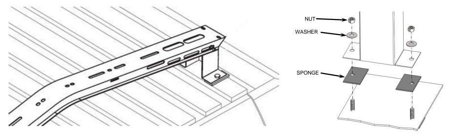
Reposition the Utility Carriers and place the (8) SPONGES between each of the MOUNTING FEET and the roof. Insert (8) 3/8" NEOPRENE WASHERS and (8) 3/8" x 1-1/2" SCREWS through each of the holes in the MOUNTING FEET from the top.
