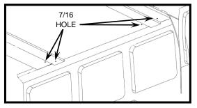
Remove the Utility Carrier to allow working space and drill eight **7/16**" diameter holes through the roof where marked. Your drilled holes should straddle the roof crossmember at the rear. At the front, one hole will fall to the front of the roof crossmember and the other hole will go through the roof crossmember.
