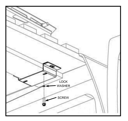
Replace the STIFFENER PLATES over the MOUNTING PLATES and secure with (2) 1/4" SPLIT LOCK WASHER and (2) 1/4"-20 X 1" HWH SCREW
