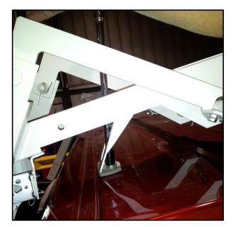
ACCESS MOUNTING HARDWARE THORUGH SLOT IN CROSSBOW
