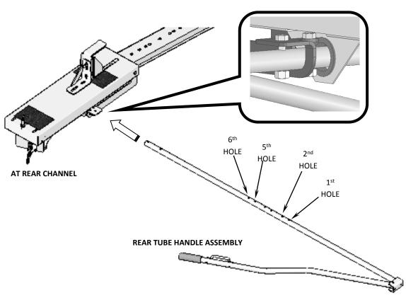
Slide **REAR TUBE HANDLE ASSEMBLY** through LH and RH Arm Grommets. At the hole locations shown, secure with (4) 5/16-18 x 1.5 Hex Head Screws and (4) 5/16-18 NyLock Nuts.
