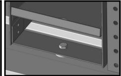
Position Manual Rack and mark to install Plusnut (SEE PAGE 4), and secure using: (1) 1/4-20 x 2-1/2 HWH Screw Grd 8 (1) Spacer (IF LOCATION FALLS IN VALLEY OF FLOOR)
