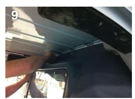
Loosely secure the floor and ceiling with the 1 ½" screws (**D**), washers (**C**), and split washers (**B**).
