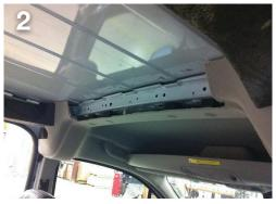
Using a knife, trim the headliner along the lower trim line between the inside edges of the outermost ceiling ribs.
