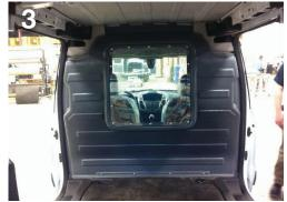
Slide the partition into place so that it lines up against the B-Pillar and along the headliner.
