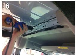
Drill pilot holes through each marked hole, then re-drill them using a 11/32" bit. You will be drilling through the van floor.
