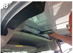
Install plus nuts (A) in the three holes in the ceiling pillar with the plus nut gun. Slide the partition into place, aligning the pre-drilled holes to the holes just drilled.
