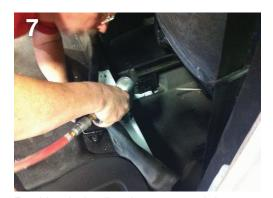
Peel back the flooring to reveal the metal underneath. Insert and secure plus nuts (A) using the plus nut gun for the four holes. Place the spacers (F) over the plus nuts before putting the flooring back in place.
