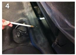
Using the four holes at the bottom of the partition as a guide, mark holes on the carpet.
