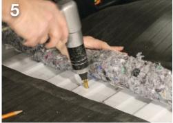
Drill the holes in the floor and B-pillar with the 11/32" drill bit. Insert the plus nuts (**A**), using the plus nut gun, in the 11/32" holes.
