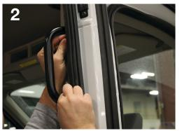
Pull back the weatherstripping around the door frame. Remove the pillar handle.
