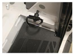
Remove the D-rings using a 1/2" nut driver.
