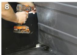
Loosely secure the sides and top of the partition with self-tapping screws (**E**), using the ¼" nut driver, in the predrilled holes. When properly positioned, tighten all bolts.
