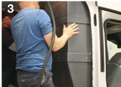
Slide the partition into place so that it lines up against the B-Pillar and along the headliner. Reattach the D-rings.
