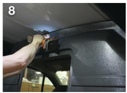
Loosely secure self-tapping screws (**F**) with the ¼" nut driver through the pre-drilled holes of the partition. When properly positioned, tighten all bolts.
