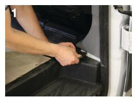
Pull back the rubber trim from around the door frame. Remove the D-rings using a 1/2" nut driver.
