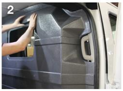
Slide the partition into place so that it lines up against the B-Pillar and along the headliner.
