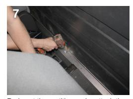
Re-insert the partition and reattach the D-rings. Loosely secure to the floor using 1 ½" screws (**E**), washers (**C**), and split washers (**D**). Loosely secure the sides of the partition with the 2" screws (**G**), washers (**C**), and split washers (**D**).
