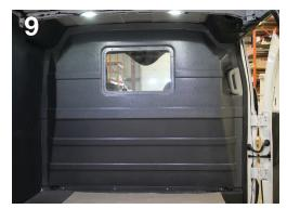
Adjust the weatherstripping. The rubber should cover the outer edge of the panel. Installation is complete.
