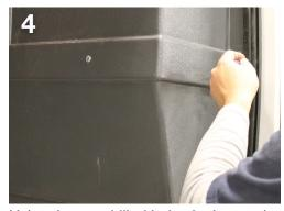
Using the pre-drilled holes in the steel rib as a guide, mark the B-pillar plastic. Mark the holes in the bottom bracket.
