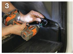
Replace the D-rings to hold the partition in the proper position.
