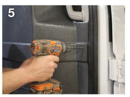
Remove the D-rings and partition. Then drill pilot holes through the plastic and the metal B-pillar.
