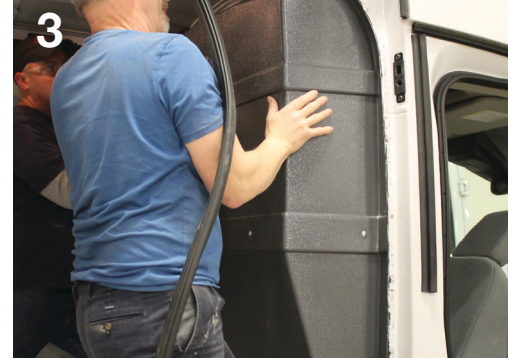
3 Slide the partition into place so that it lines up against the B-Pillar and along the headliner. Reattach the D-rings.
