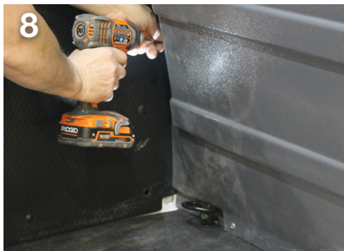
8 Loosely secure the sides and top of the partition with self-tapping screws (E), using the 1/4" nut driver, in the pre-drilled holes. When properly positioned, tighten all bolts.
