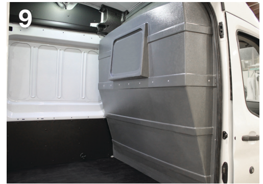
9 Adjust the weatherstripping along the door frames. The rubber should cover the outer edge of the panel. Installation is complete.
