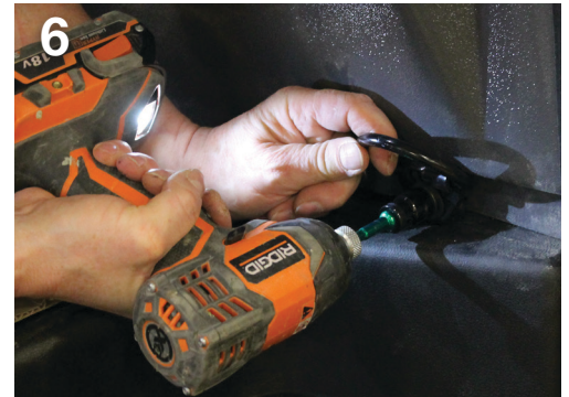
6 Slide the partition into place and reattach the D-rings.
