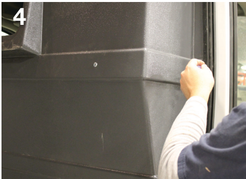
4 Mark the holes at the top of the partition, on the bottom bracket and in the partition at the end of the steel rib on the B-pillars. Remove the D-rings once more and remove the partition.
