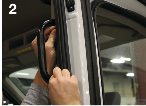
2 Pull back the weatherstripping around the door frame. Remove the pillar handle.
