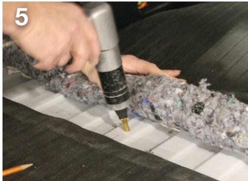
5 Drill the holes in the floor and B-pillar with the 11/32" drill bit. Insert the plus nuts (A), using the plus nut gun, in the 11/32" holes.
