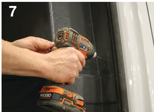
7 Loosely attach the partition with the 1 1/2" Philip screws (D), flat washers (B), and split washers (C) to all areas where plus nuts were installed in step 5.
