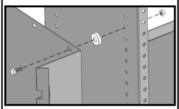
Align holes in Spool Carrier with holes along right hand side of Upright and secure using:
